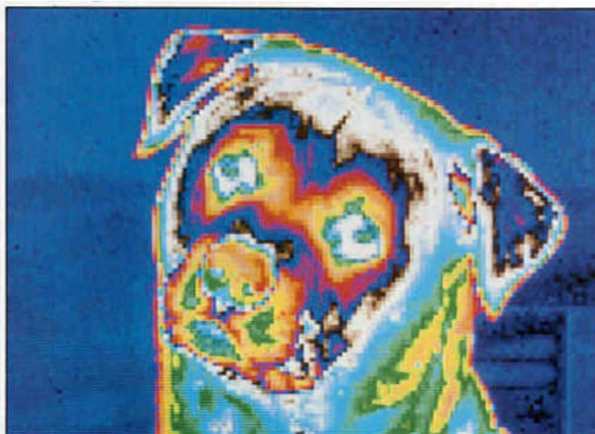
*This infrared image of a prize-winning Rottweiler was recorded by an Amber 128 × 128 indium antimonide staring focal plane array. After it was recorded, the image was photographed from a display generated by Amber's Pro-View imaging system. Photo courtesy of Amber, a Raytheon Co., of Goleta, Calif.* □
