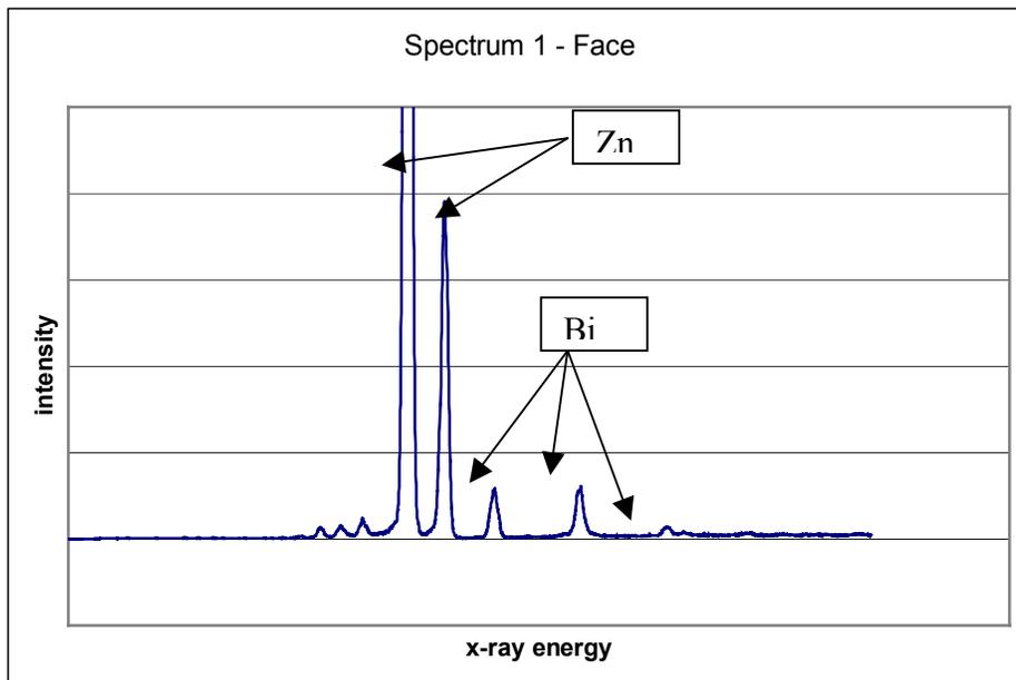
By far the most prominent peak in this spectrum is Zn (exceeding full scale in the plot above by a factor of 5). Other constituents include Bi (marked) and Fe, Co, and Ni (the three peaks to the left of Zn). A similar x-ray spectrum taken from the dark, fractured cylindrical
