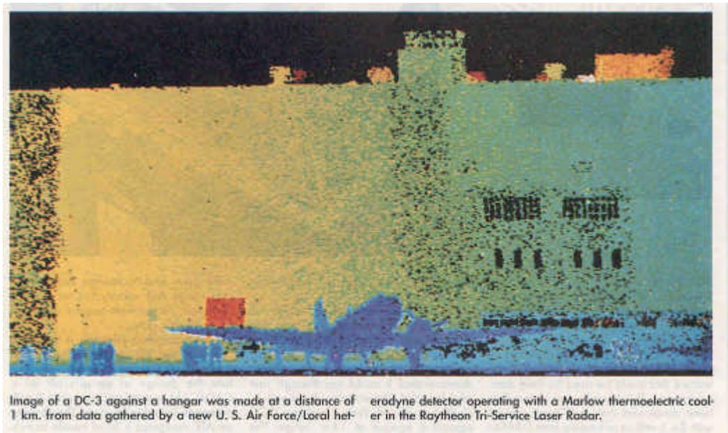
Image of a DC-3 against a hangar was made at a distance of 1 km. from data gathered by a new U. S. Air Force/Loral heterodyne detector operating with a Marlow thermoelectric cooler in the Raytheon Tri-Service Laser Radar.
